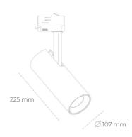
COB 3000 [K] HI EFFICIENT Light colour CRI 90 Led chip flux 5523 [lm] Luminous flux 4970 [lm] System power 34 [W] Luminaire Efficiency 146 [lm/W] Beam angle 45° Controller ON/OFF MacAdam 3 SDCM
